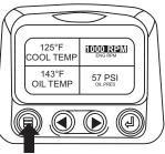
15. Touch the "Menu Button" to exit the Main menu and return to the engine parameter display.
